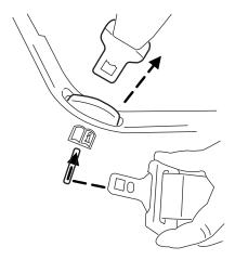
2. Find the clips attached near the ends of the lap/shoulder belts.
